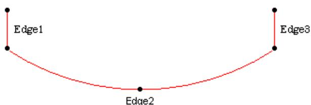
However, the *TopoDS* package provides only the data structure of the topological entities. Algorithm classes available to compute standard topological objects can be found in the *BRepBuilderAPI* package. To create an edge, you use the *BRepBuilderAPI\_MakeEdge* class with the previously computed curves:
