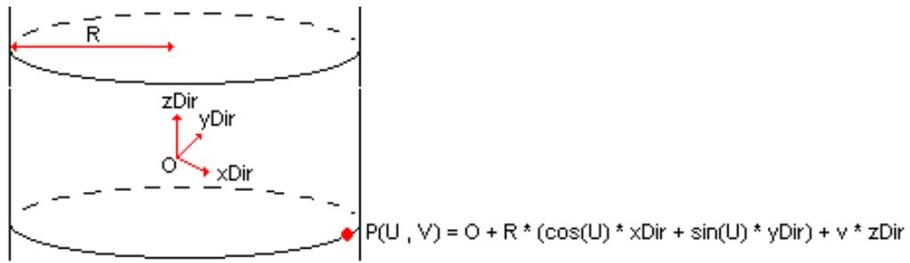
The advantage of having such parameterized geometries is that you can compute, for any (U, V) parameters of the surface:
