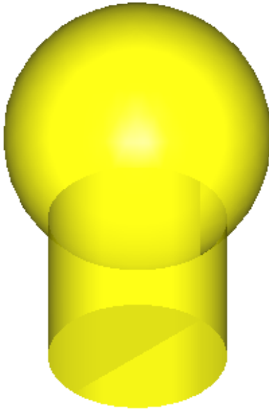
Figure 53: The result of FUSE operation between cylinder and sphere
