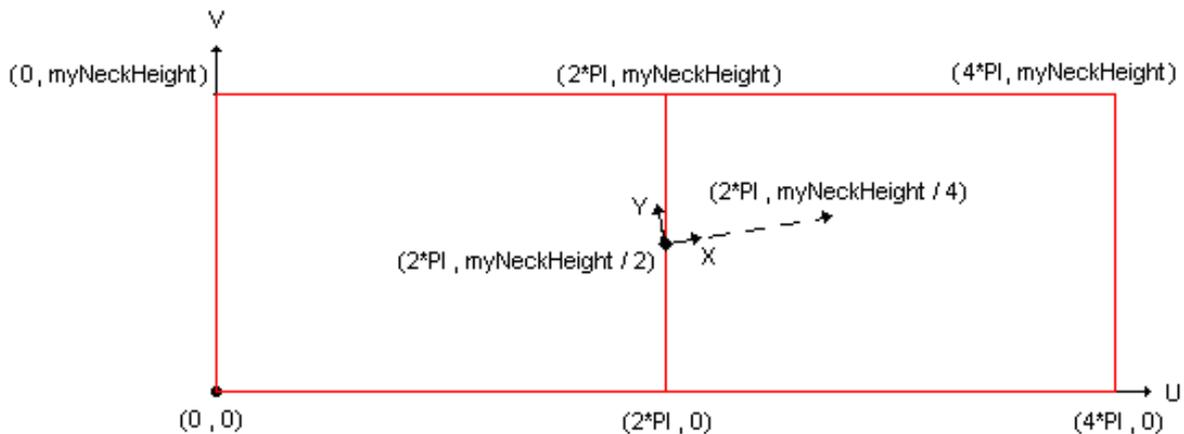
To use 2D primitive geometry types of Open CASCADE Technology for defining a point and a coordinate system, you will once again instantiate classes from gp:
