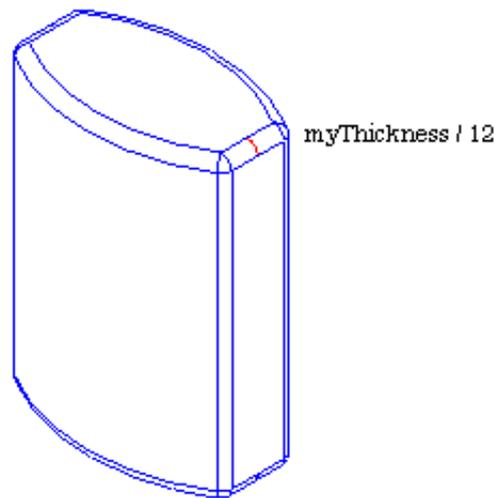
To apply fillets on the edges of a shape, you use the *BRepFilletAPI\_MakeFillet* class. This class is normally used as follows:
