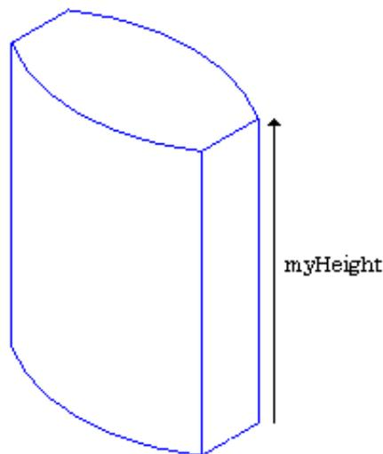
Your current profile is a wire. Referring to the Shape/Generates table, you need to compute a face out of its wire to generate a solid. To create a face, use the *BRepBuilderAPI\_MakeFace* class. As previously explained, a face is a part of a surface bounded by a closed wire. Generally, *BRepBuilderAPI\_MakeFace* computes a face out of a surface and one or more wires. When the wire lies on a plane, the surface is automatically computed.
