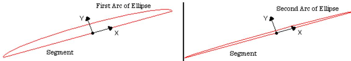
You have already used the *Geom* package to define 3D geometric entities. For 2D, you will use the *Geom2d* package. As for *Geom*, all geometries are parameterized. For example, a *Geom2d\_Ellipse* ellipse is defined from:
